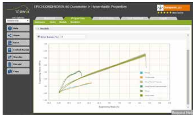
Using Matereality's Viewer module to quantify the goodness of fit of a hyperelastic equation to raw data.
