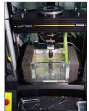
Saline cell to measure properties for 'in-vivo' applications.
