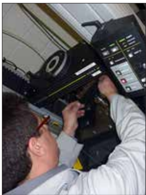
Loading test specimens for a plate-twist shear modulus test.
