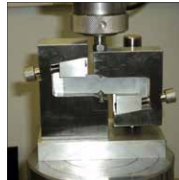
Measuring shear properties of composites using digital image correlation (DIC).
