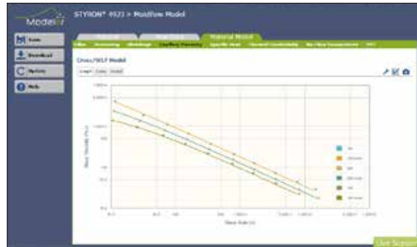
Using Matereality's CAE Modeler software to create a Moldflow *.UDB file.
