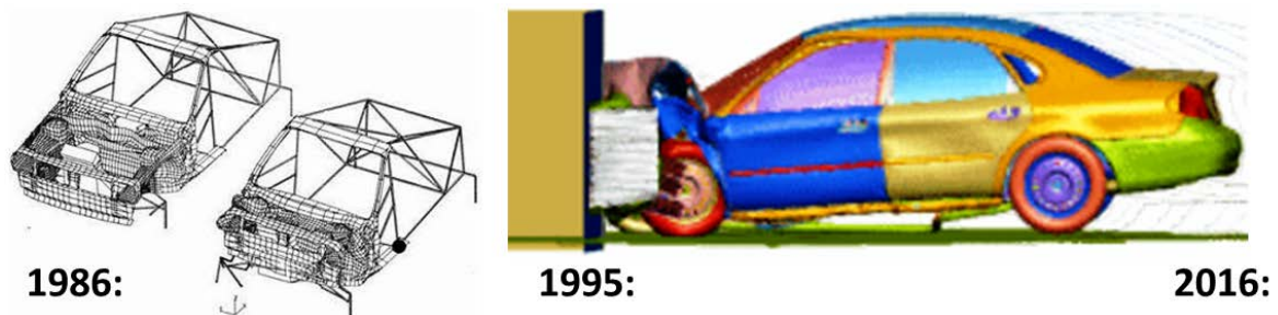
Fig.2: Increased computational power has resulted in FEM models with more elements and details.
