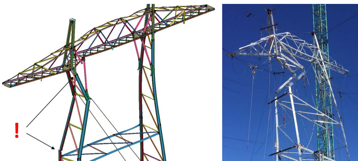
Fig. 15: The explicit solver may predict the collapse that take place just after the capacity is meet.
