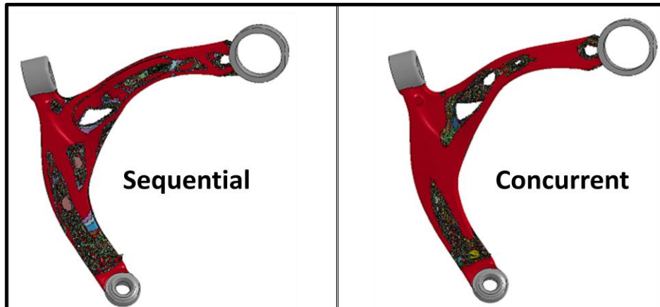
Fig.8: Resulting deformed structures of trade-off from running the sequential topology optimization of stiffness and energy absorption (left), and concurrent scaled weighting topology optimization, resulting from an equal preference of compliance and energy absorption (right).
