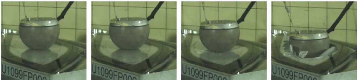
Fig.1: Image series of a head impact on automotive side window out of PMMA with t = 4 mm [4]
