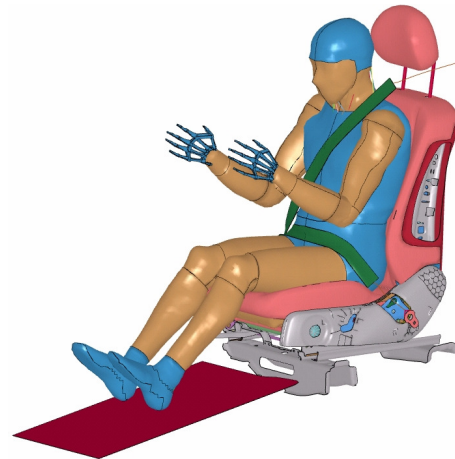
Figure 14: AM50-THUMS in seat model (courtesy of DaimlerChrysler AG)
