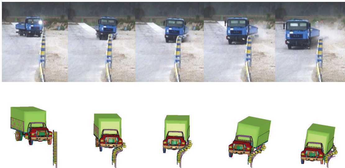
Figure 7: The barrier deformation during TB42 test (top – experiment; bottom – simulation)
