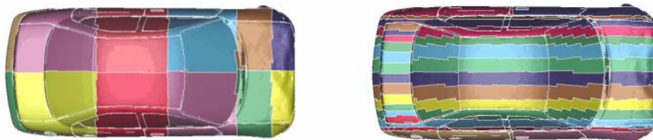
Figure 1. LS-DYNA Decomposition Results for Default (left) and Modified (right) RCB
