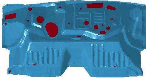
Trimmed-out Holes Filled with LS-PrePost
