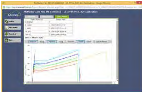
Figure 4. CAE Modeler for LS-DYNA is used to create a MAT024 material card.
