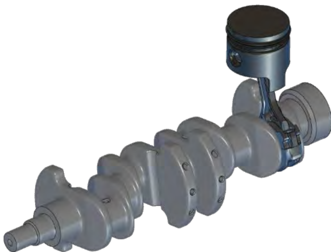
Figure 5. Left image: The crankshaft assembly consists of the crankshaft, conrod, piston pin and piston. Right image: The assumed cylinder pressure curve.
