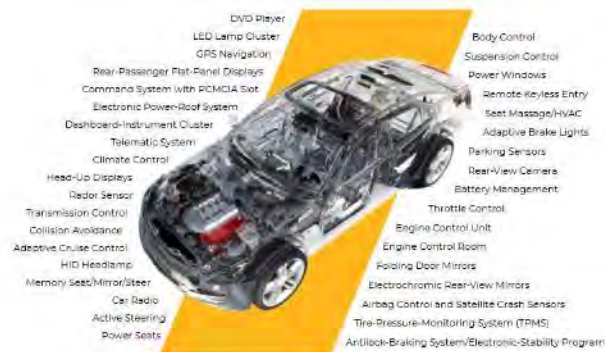
Electronics in the modern automobile
