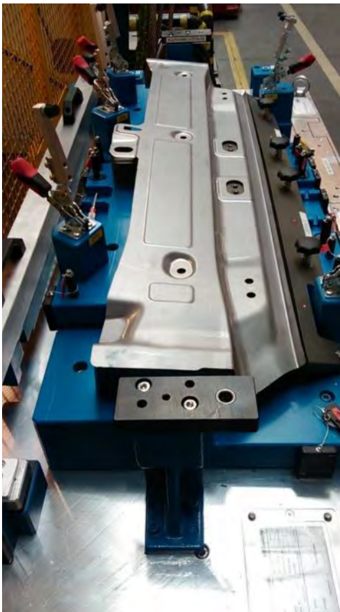
Checking part on controlling devices on the shop floor
