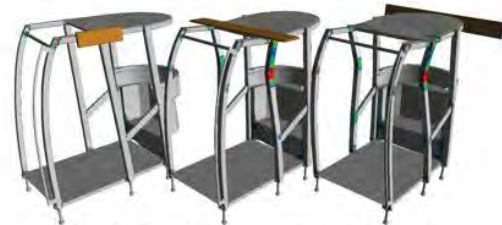
RollOver Protection Structure
