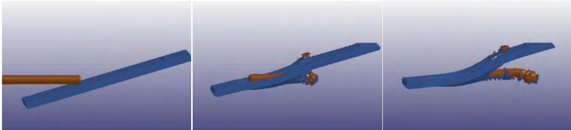
Projectile penetrating steel plate
