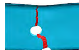
Ductile cracking in shell
