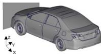
Fig. 2 Car crash FE model
