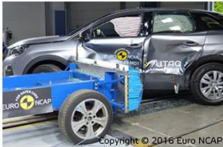
New Peugeot 3008 side crash Euro NCAP test and FE model
