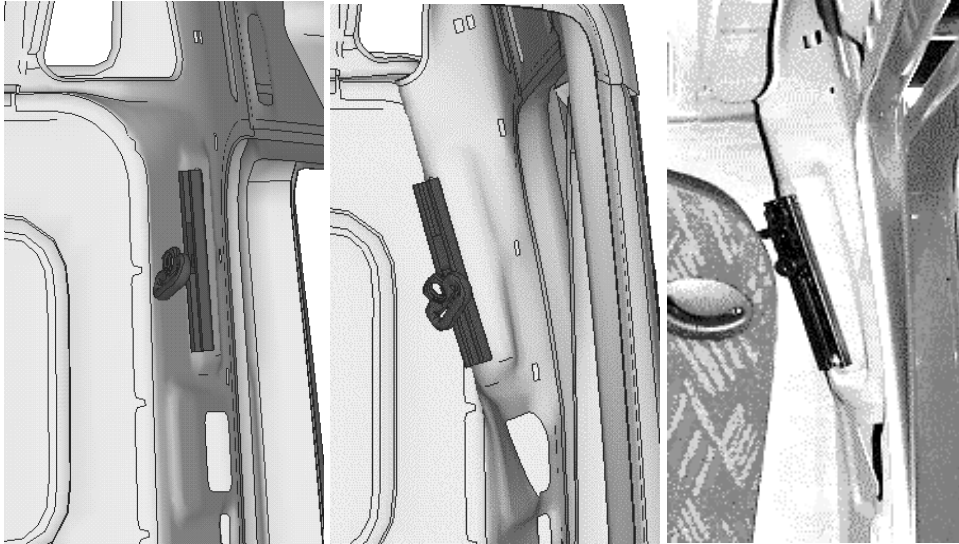
Figure 3 Undeformed state and comparison between LS-Dyna simulation results and experimental results for the FMVSS test
