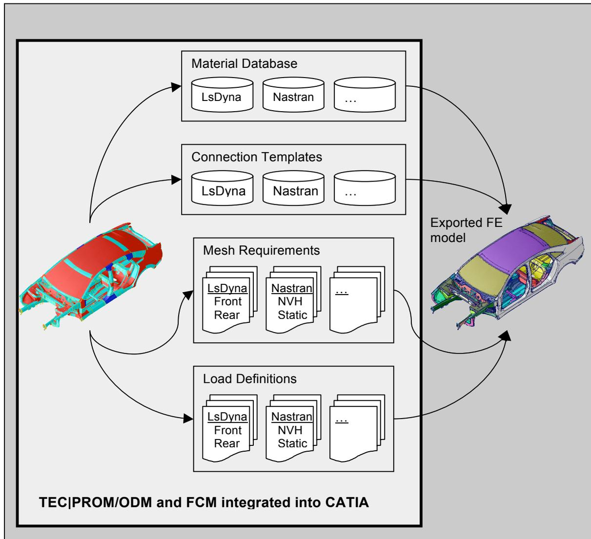
Picture 4: The Fast Concept Modeling (FCM) tool
