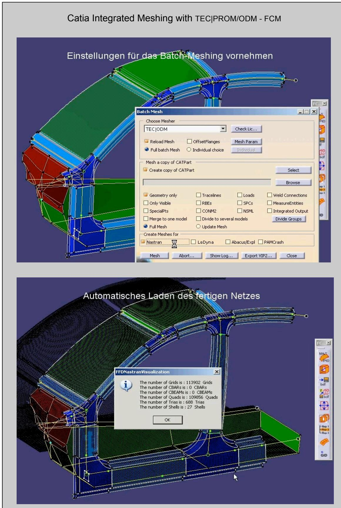
Picture 7: CATIA V5 integrated meshing with TEC|ODM
