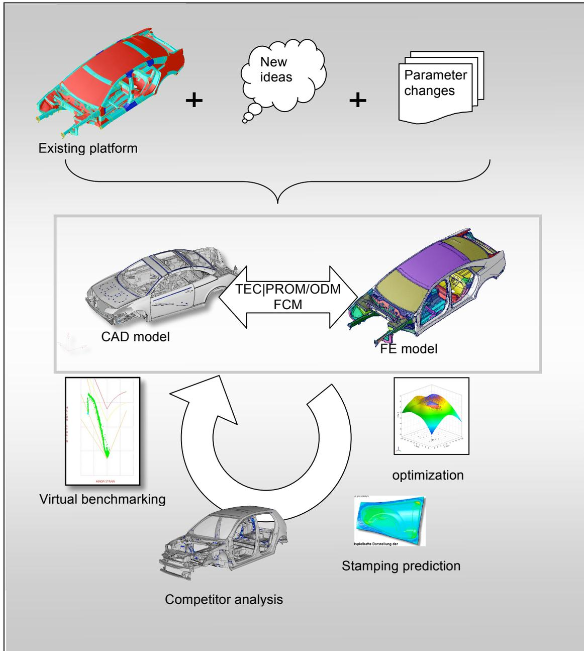
Picture 1: Process overview of a design modification
