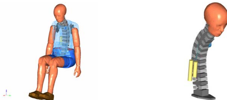
Fig. 9: BioRID-II FE Quality dummy model (left) and a detail of the spine column (right)
