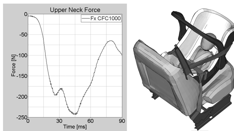
Figure 11: Q0 in a infant carrier and results of a frontal impact.
