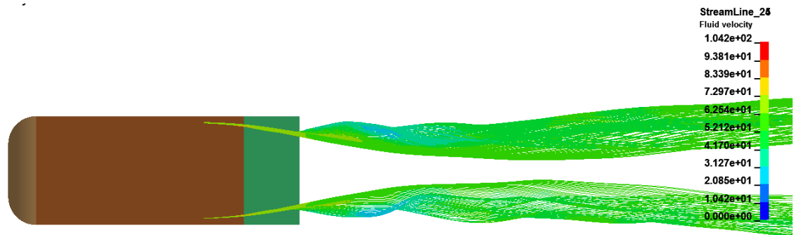
Figure 10: Streamlines highlighting the two side vortices that start close to the edge and move inwards.
