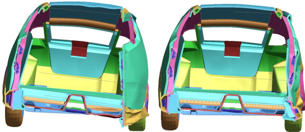
Fig.22: TARF-LCV Optimized design: Pole Impact(left) and Side Impact(right)
