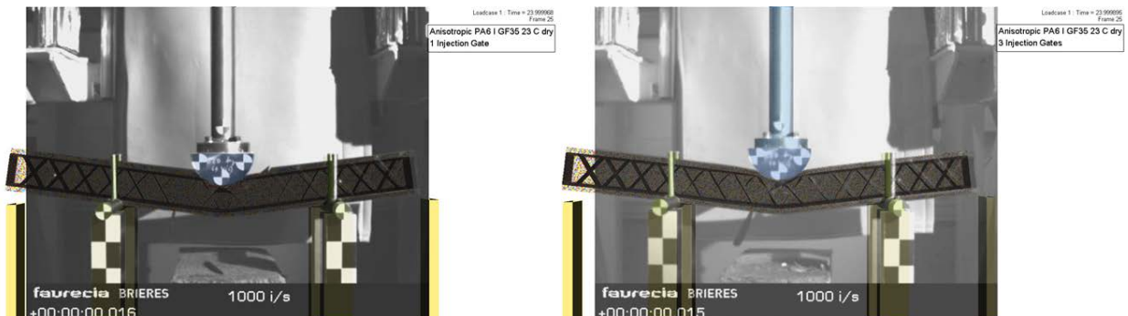
Fig.8: Dynamic three points bending superposition Test / Simulation 1 injection gate (left), 3 injection gates (right)
