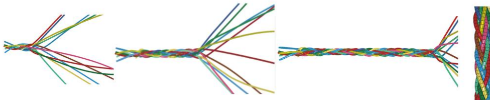
FE-Simulation of a braiding process
