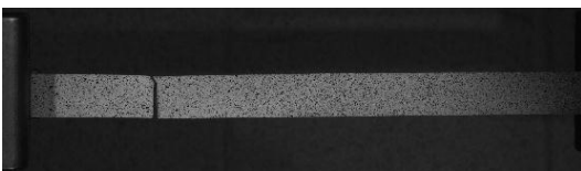
Figure 12. Major strain of DP780 in the rolling direction.
