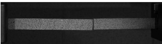
Figure 10. Major strain of DP780 along transverse direction.
