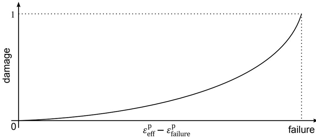
**Figure M81-2.** A nonlinear damage curve is optional. Note that the origin of the curve is at (0,0). It is permissible to input the failure strain EPPF as zero for this option. The nonlinear damage curve is useful for controlling the softening behavior after the failure strain is reached.
