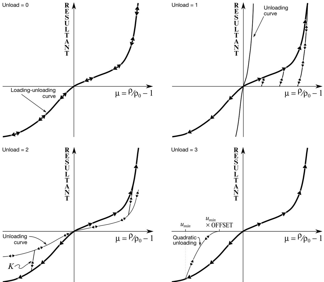
Figure EOS15-1. Load and unloading behavior.
