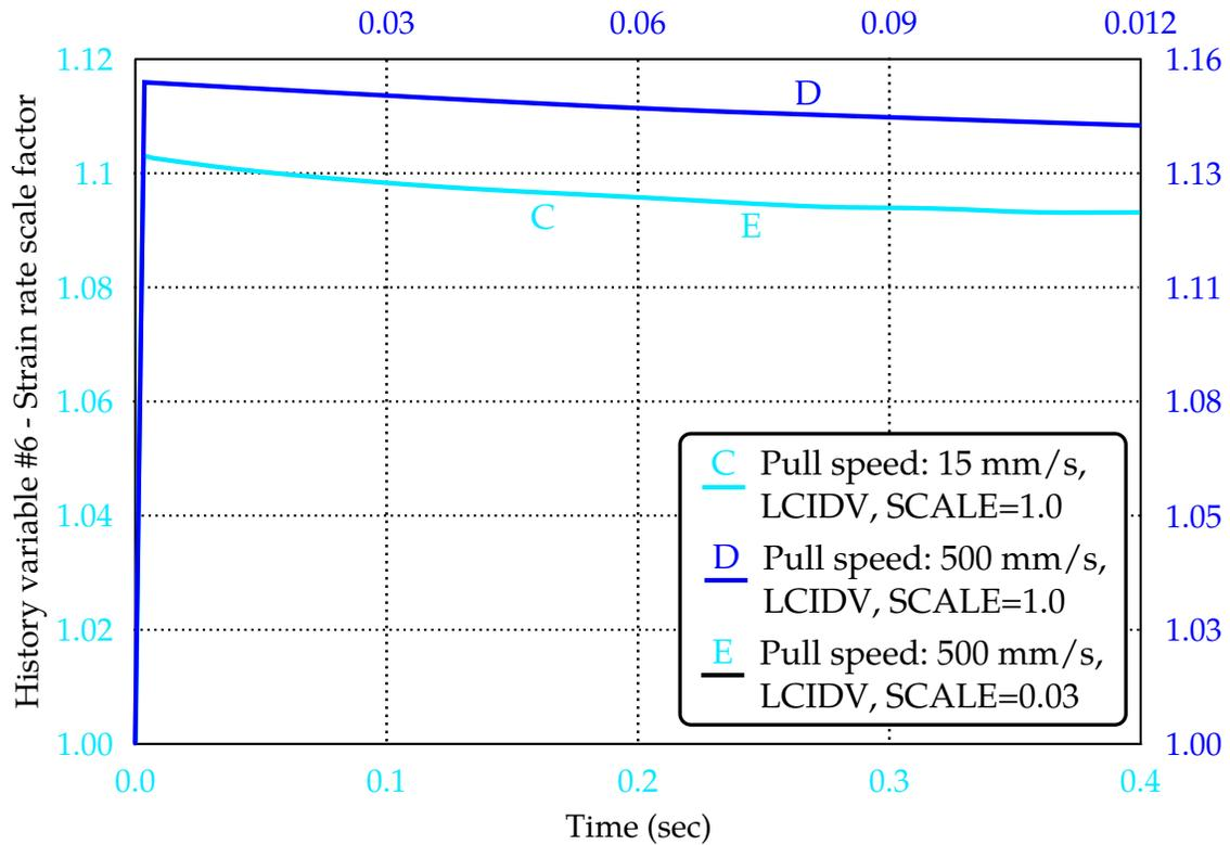
**Figure M260A-4.** Recovered strain rate scale factors under various conditions shown.
