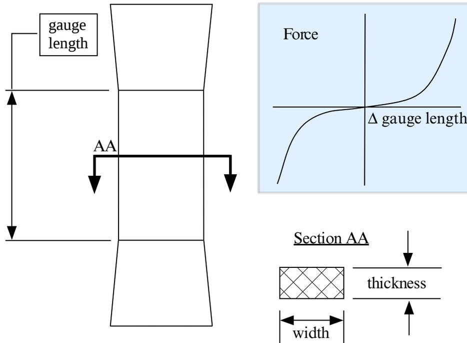
Figure M218-1. Uniaxial specimen for experimental data
