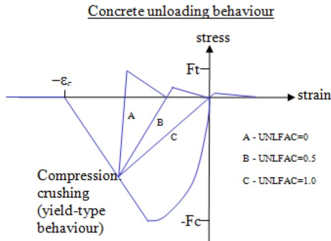
**Figure M172-4.** Concrete unloading behavior
