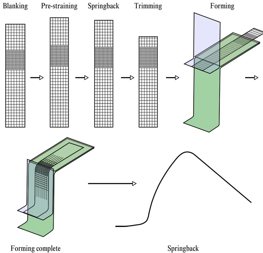
Figure M125-4. NUMISHEET 2011 Benchmark #4 simulation procedure.
