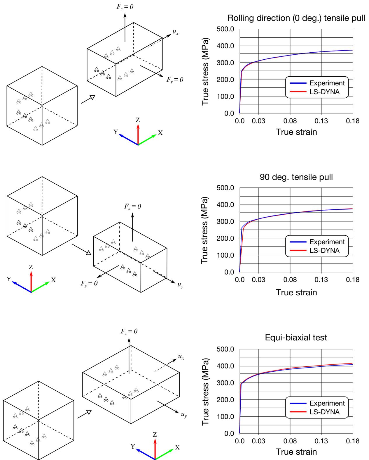
Figure M122-1. Validation with experiments - BM1 NUMISHEET 2011
