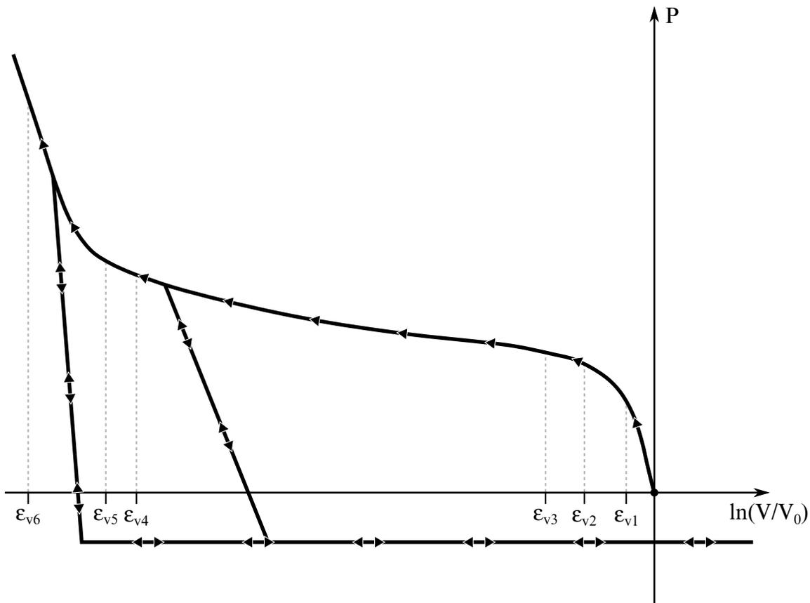
**Figure EOS8-1.** Pressure versus volumetric strain curve for Equation of state Form 8 with compaction. In the compacted states the bulk unloading modulus depends on the peak volumetric strain. Volumetric strain values should be input with correct sign (negative in compression) and in descending order. Pressure is positive in compression.
