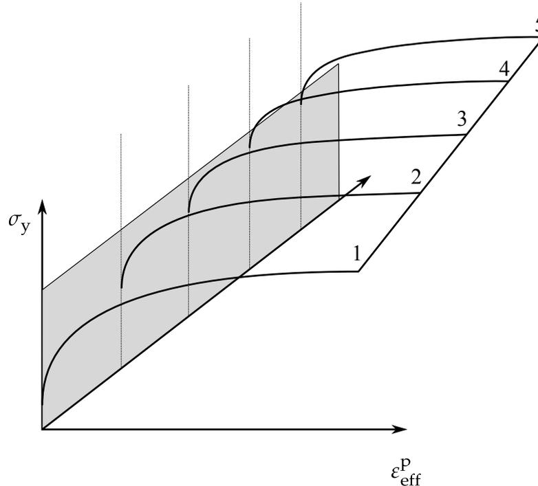
**Figure M24-1.** Rate effects may be accounted for by defining a table of curves. If a table ID is specified a curve ID is given for each strain rate, see \*DEFINE\_TABLE. Intermediate values are found by interpolating between curves. Effective plastic strain versus yield stress is expected. If the strain rate values fall out of range, extrapolation is not used; rather, either the first or last curve determines the yield stress depending on whether the rate is low or high, respectively.
