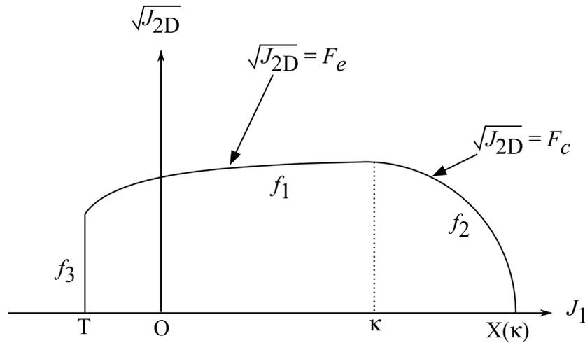
**Figure M25-1.** The yield surface of the two-invariant cap model in  $\sqrt{J_{2D}} - J_1$  space. Surface  $f_1$  is the failure envelope,  $f_2$  is the cap surface, and  $f_3$  is the tension cutoff.
