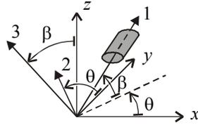
**Figure M235-1.** Yarn orientation schematic.
