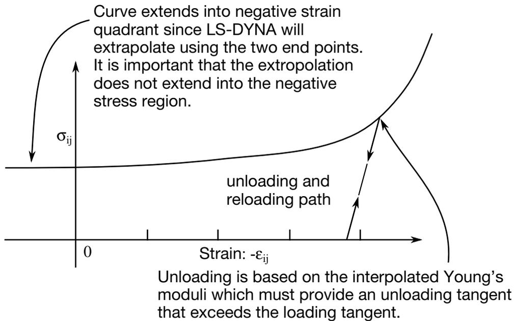
**Figure M126-1.** Stress versus strain. Note that the “yield stress” at a strain of zero is nonzero. In the load curve definition the “time” value is the directional strain and the “function” value is the yield stress. Note that for element types 0 and 9 engineering strains are used, but for all other element types the rates are integrated in time.
