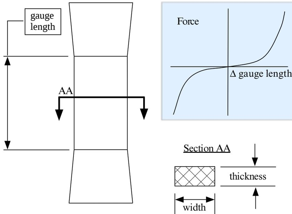
**Figure M27-1.** Uniaxial specimen for experimental data
