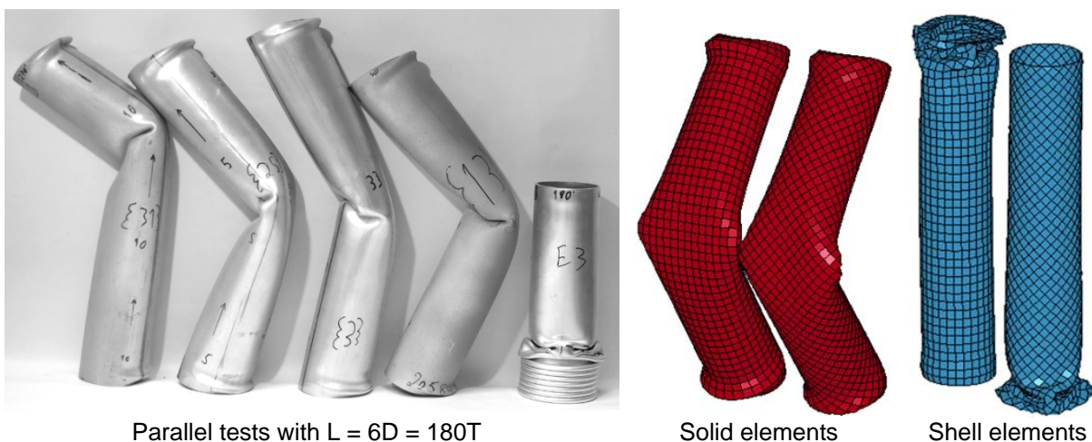
Fig.2: The experiments confirm a sensitive case as captured by the solid elements.
