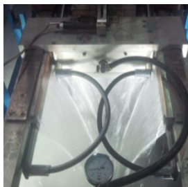
Fig.1: Water flow in a CC mould
