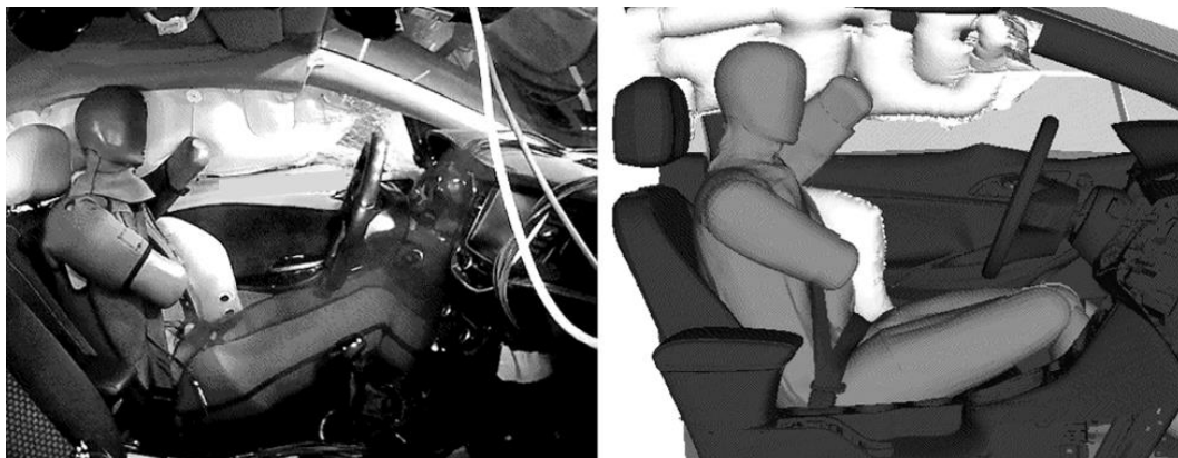
Fig.3: Analysis of WorldSID-50 Dummy Kinematics Test vs. Simulation in AE-MDB Side Impact
