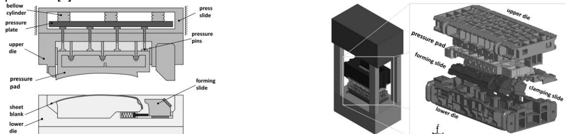
Fig. 1: Left: Principle model of a deep drawing tool according to. [2] Right: FEM model of the deep drawing tool with an exploded view. [3]
