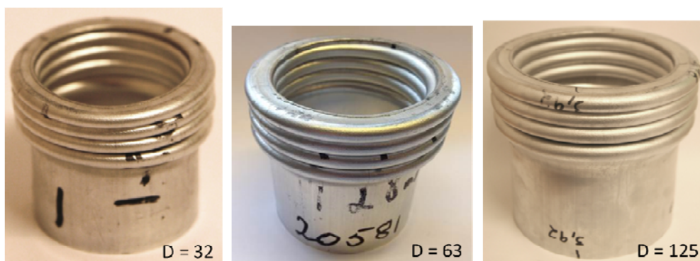
Fig. 1: Tests with L = 2D = 60T shows the same deformation mode independent of the scale.
