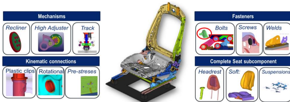
Fig.1: Typical connections for car seat.
