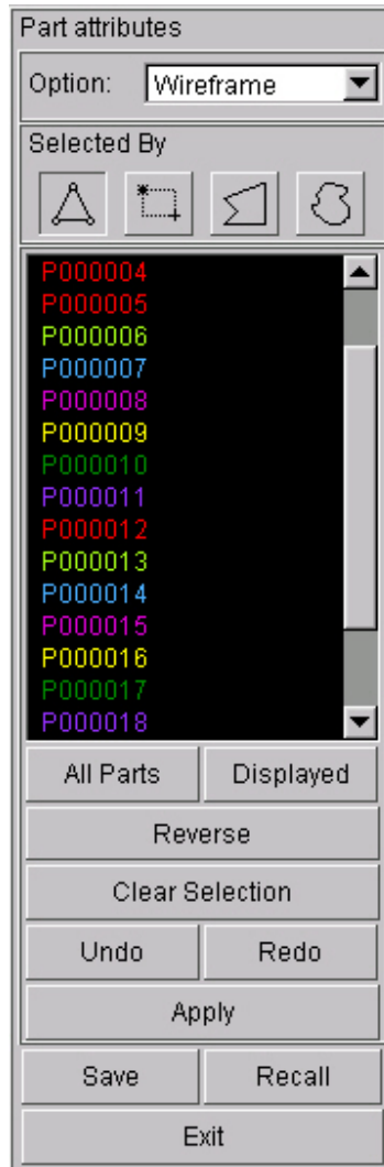
Figure 4.7.4 Part Attributes control window (Wire Frame)
